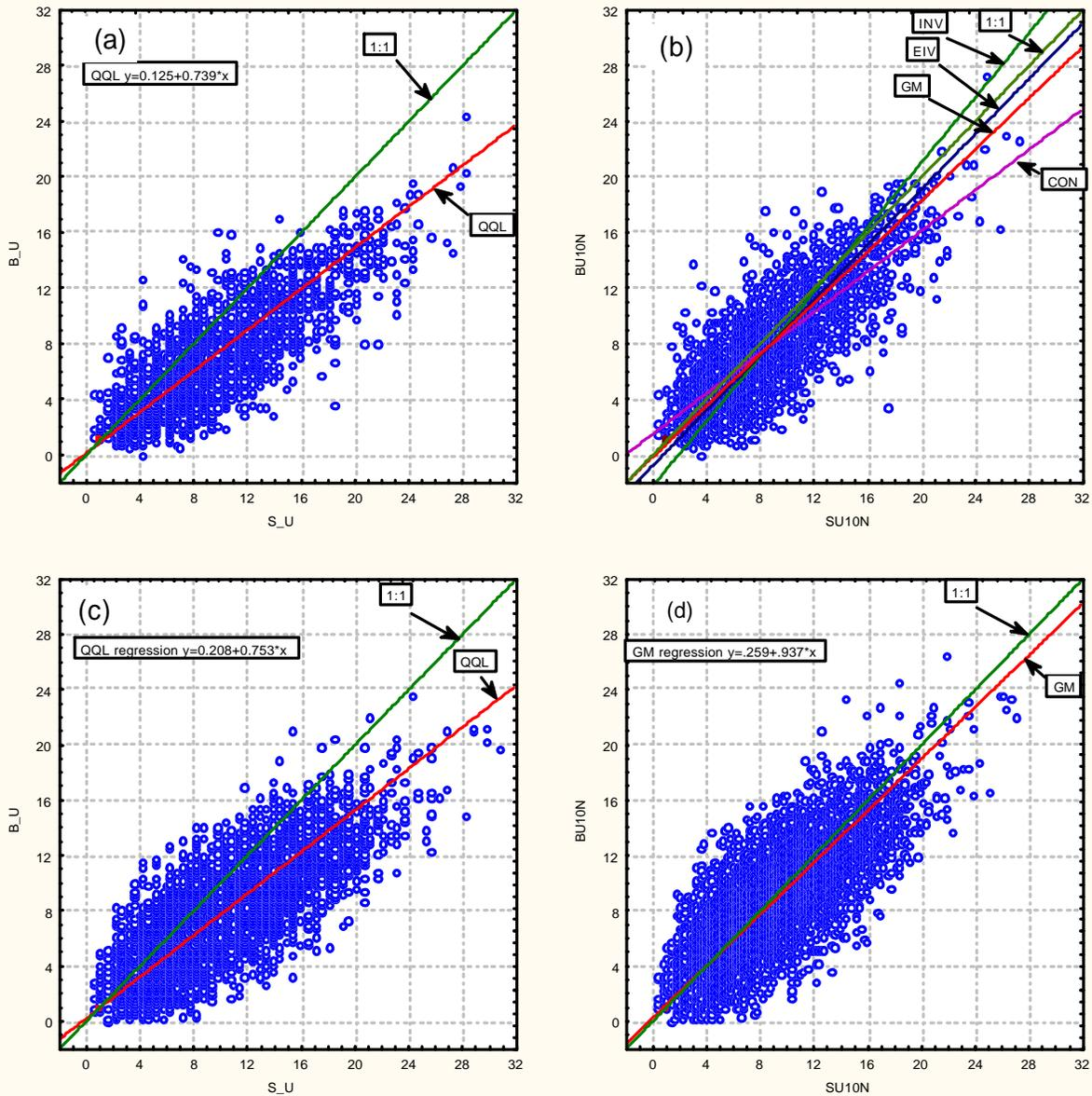
**Figure 2 Scatterplots for buoy on measured ship wind speeds, with 1:1 and neutral regression lines a) east coast original, b) east coast BU10N on SU10N also with inverse, EIV, and conventional regression lines, c) west coast original, d) west coast BU10N on SU10N.**
