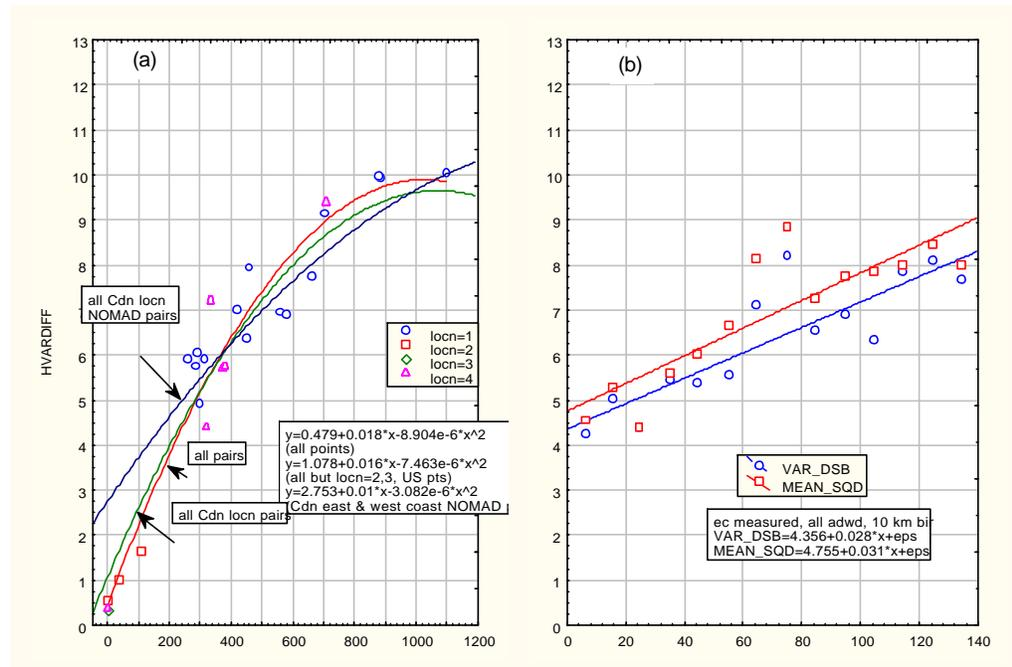
**Figure 1 (From TS03) Variograms to determine buoy and ship observational error variance: a) half variance of difference for each buoy-buoy pair, vs separation distance of buoy-buoy pairs, with 2<sup>nd</sup> order polynomial best fit lines; b) variance of difference for binned differences of east coast measured adjusted ship-buoy pairs vs separation distance, also mean of squared differences for binned differences, with linear best fit lines.**
