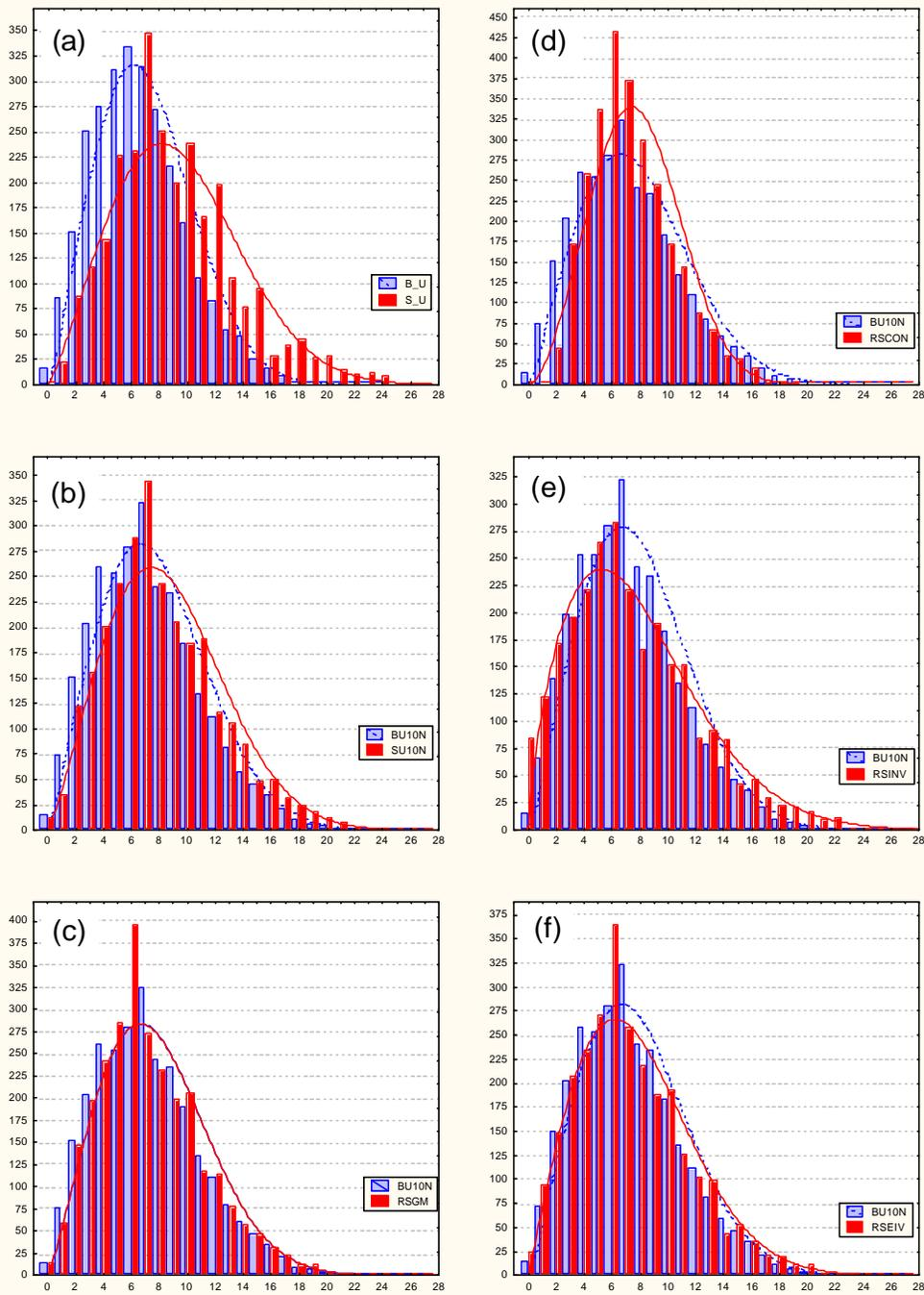
**Figure 5** Frequency distributions of east coast measured paired ship and buoy wind speeds, fitted to Weibull distribution a) original buoy and ship b) BU10N and SU10N, c)-f) BU10N and regressed SU10N winds, converted using: c) geometric-mean, d) conventional, e) inverse, and f) EIV regression equations.
