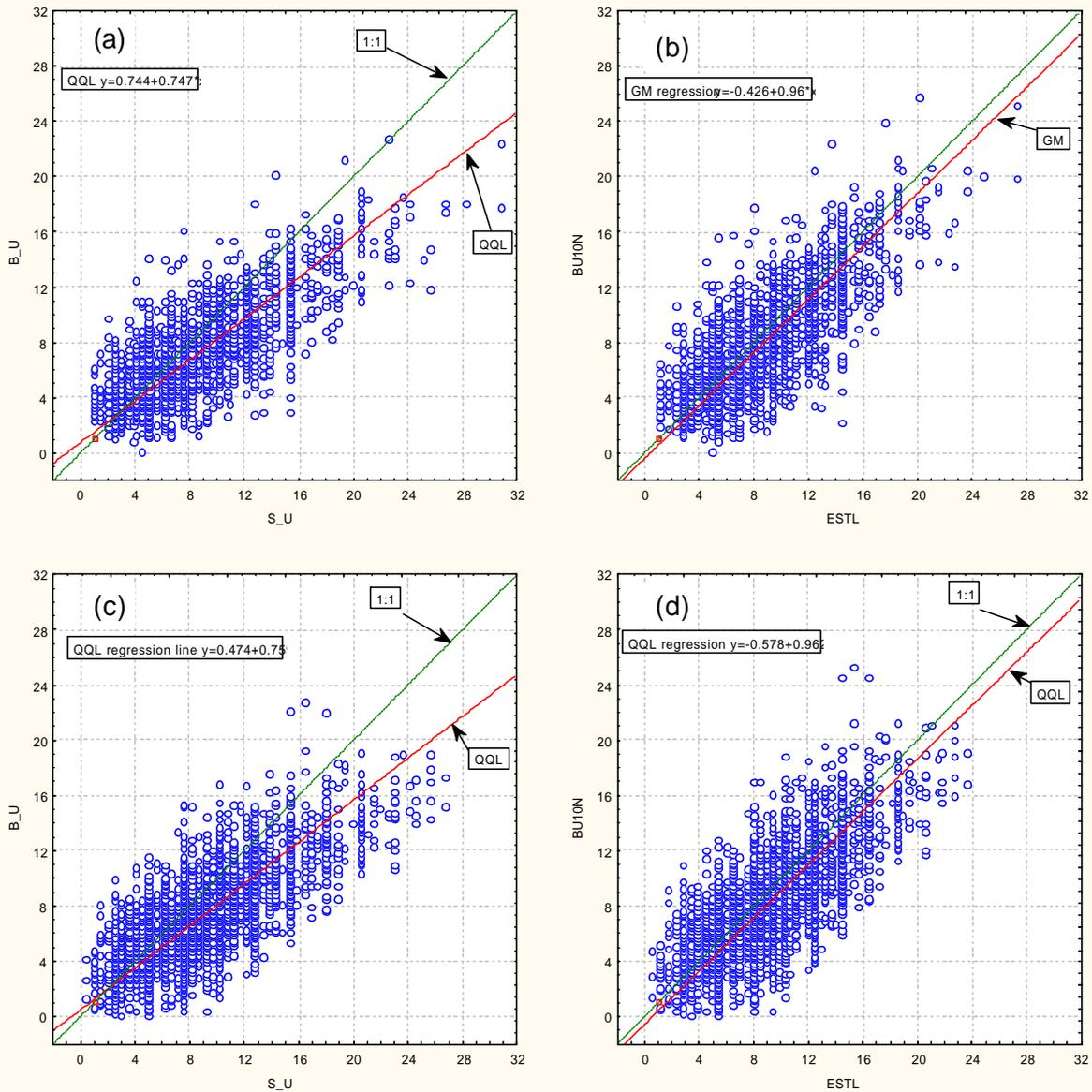
**Figure 3 Scatterplots for buoy on estimated ship wind speeds, with 1:1 and neutral regression lines a) east coast original b) east coast BU10N on UEL, c) west coast original, d) west coast BU10N on UEL.**
