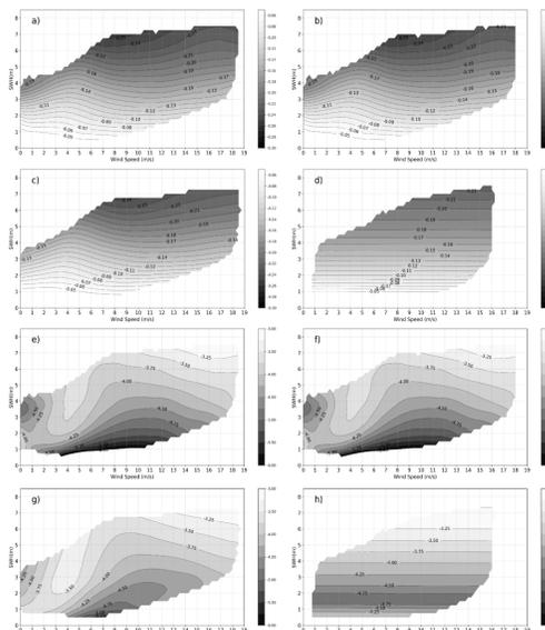
**Fig. 3:** a,b,c,d) - isolines for the global SSB (m) from bin-averaging into boxes 0.25 m/s by 0.25 m over the ( $H_s, U_{10}$ ) domain. a) - J3, cycles 70-105, b) - J2, cycles 18-55; c) - J-1, cycles 257-294; d) - SA cycles 116-124 (cf. Vandemark et al., 2002, Fig.1); e,f,g,h) - isolines for normalized value  $SSB=H_s$  (in percents) over the ( $H_s, U_{10}$ ) domain for the same data.
