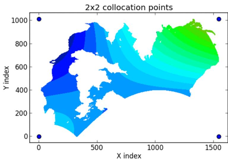
Bottom roughness estimation after 93 iterations
