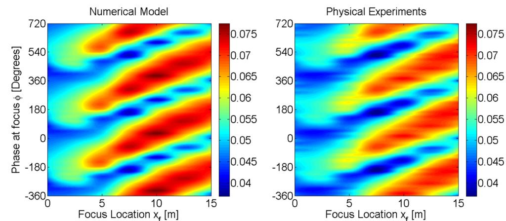
Maximum runup elevation at each focused wave amplitude
