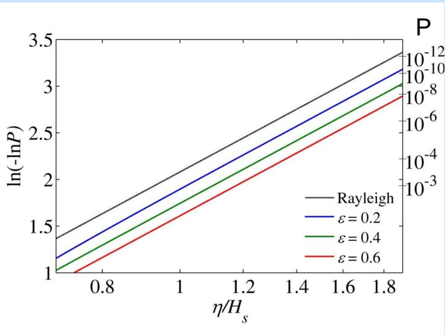
Rogue wave occurrence in a non-stationary record of two equal length parts (coloured lines) is much higher than if the record were treated as 2 stationary parts (black).
