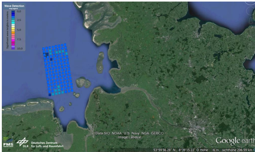
Fig.10: NRT-processing example for TerraSAR-X acquired on 22.11.2015 at 17:10 UTC over German Bight. For the common users, a file with the data (lon, lat, H_s ), the Google Earth file (.kmz) to preview the image file (.jpg) with color-coded wave heights are provided.
