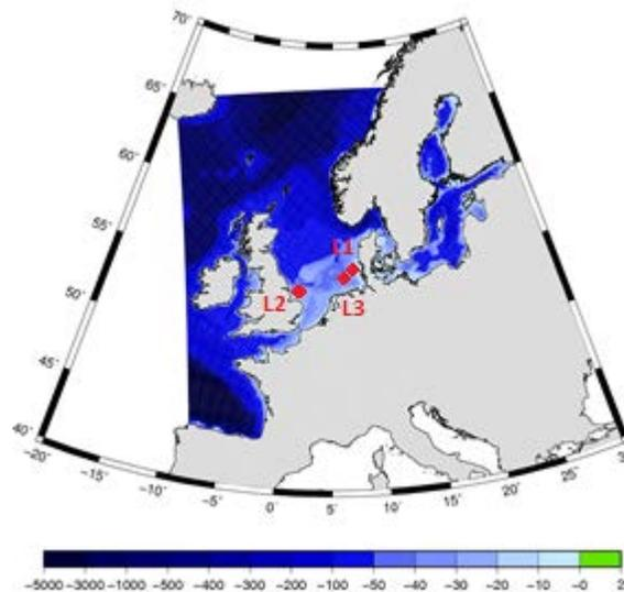
**Fig. 1** Model domain and bathymetry for hydrodynamic model TRIM-NP and locations selected for more detailed analysis.
