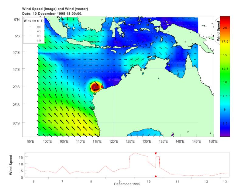
Blended wind field for Tropical Cyclone Frank (1995) when the NCEP vortex was removed using the modified Kurihara et al. method
