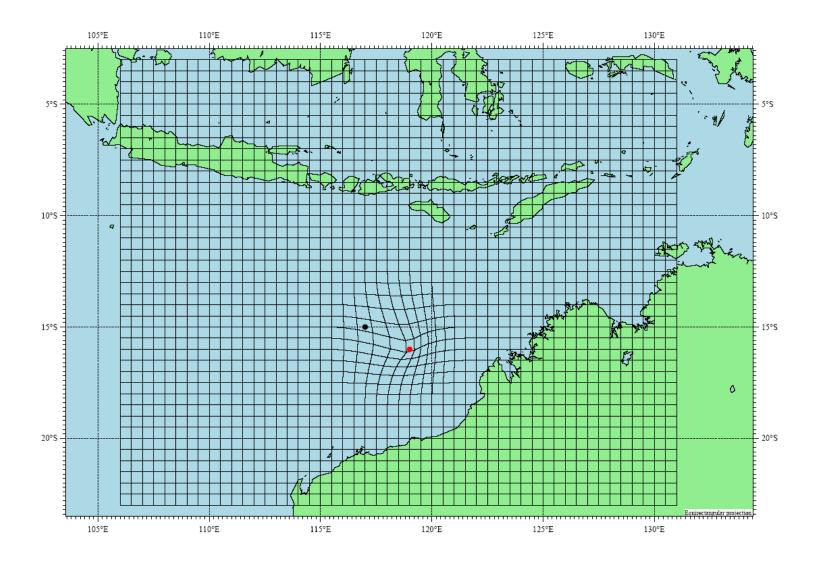
Example of a grid distorted using the vortex relocation method
