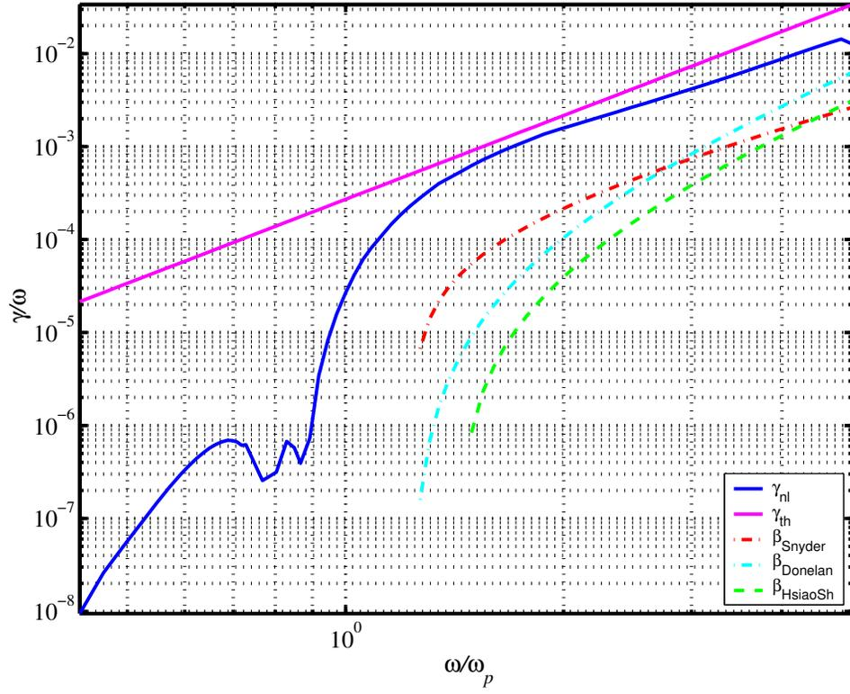
Figure 7:  $\Gamma_k$  compared with different models for  $S_{in}$
