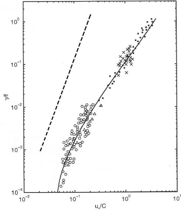
Figure 3: Comparison of experimental data for the wind-induced growth rate  $2\pi \gamma_{in}(\omega)/\omega$  taken from [2] and the damping due to four-wave interactions  $2\pi \Gamma(\omega)/\omega$ , calculated for narrow in angle spectrum at  $\mu \simeq 0.05$  using Eq. (1) (dashed line)
