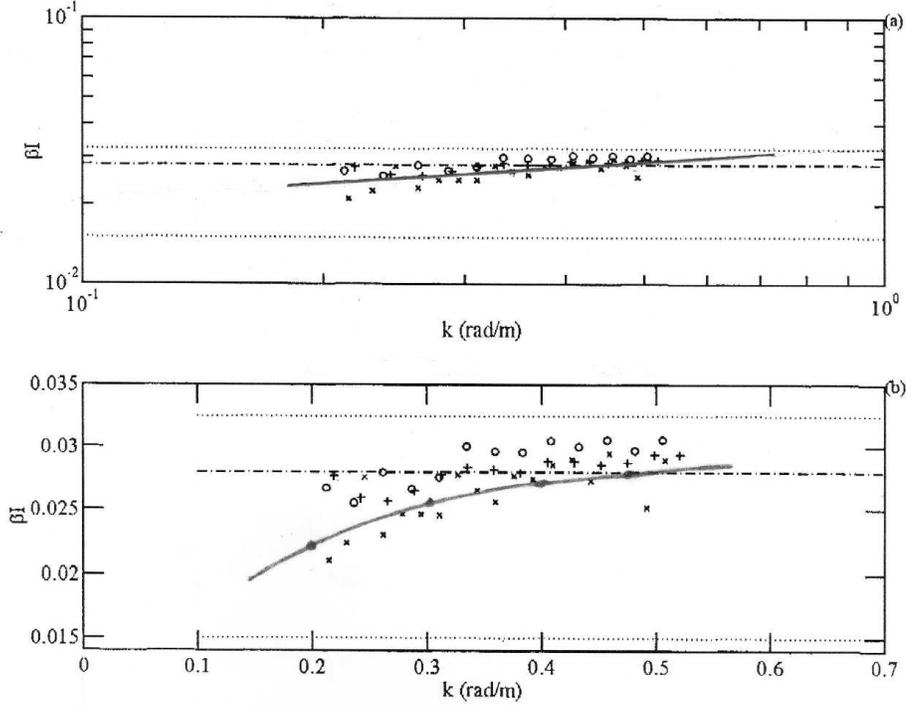
Figure 2: Dimensionless wavenumber spectral coefficient  $\beta_i$  plotted in logarithmic scales (a) and linear scales (b), taken from [1]. Here crosses represent omnidirectional (averaged by angles) spectrum and dots correspond to  $\xi(k) = 2\beta_I u_* g^{-0.5} k^{-2.5}$ . The solid line on (a) and solid curve on (b) correspond to  $\xi(k) \simeq k^{-7/3}$ .
