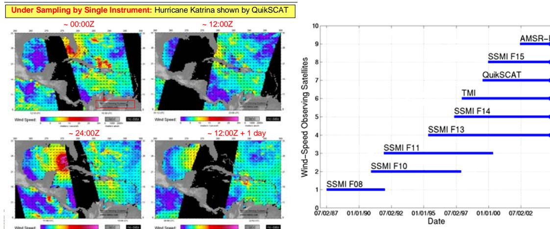
**Figure 1:** Left – QuikSCAT sampling around 28 August 2005 (from Remote Sensing System, Inc, <http://www.remss.com/>). Note it only partially sampled Hurricane Katrina about once per day. Right - Timelines of the long-term satellites that observe sea surface wind speeds.
