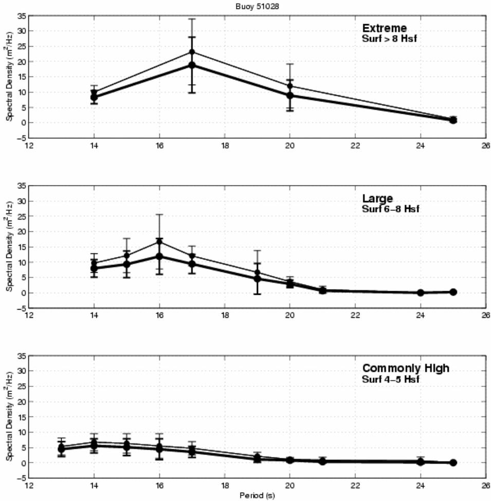
Figure 7. Buoy 51028 composite mean and standard deviation for extreme, large, and commonly high surf categories for the H3 (thin lines) and H12 (thick lines).
