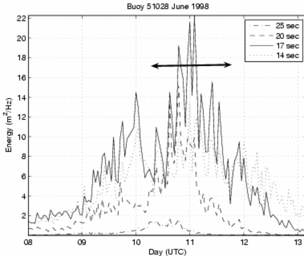
Figure 5. 8-12 June, 1998 NDBC buoy 51028 spectral density (energy). The double arrow denotes a 36-hour period chosen as the episode maximum.
