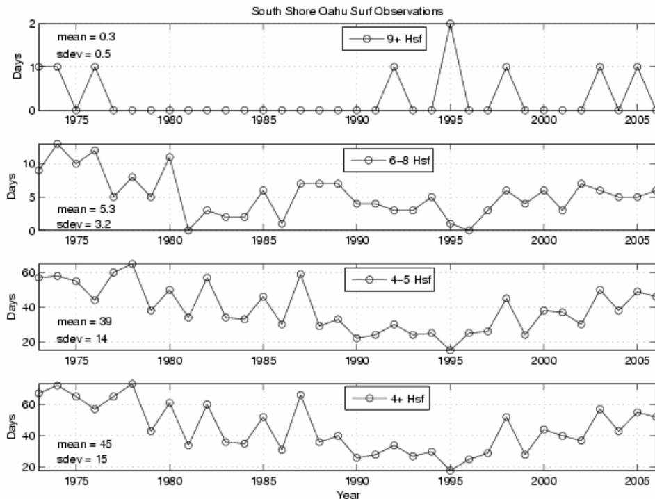
Figure 4. Year-to-year variations of the number of days of surf per year in the surf height categories from top to bottom, respectively: **extreme** (>8 Hsf or 5 m), **large** (6-8 Hsf or 3.5-5m), **commonly high** (4-5 Hsf or 2.5-3m), and commonly high or greater. The mean and standard deviation (sdev) of each are given.
